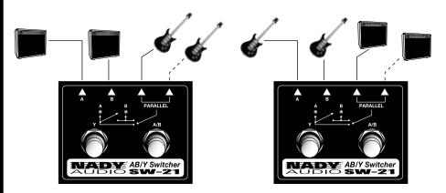
Switch between two amps or send to both amps simultaneously
